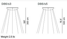
NOTE: The final shape of the luminaire may vary according to the length of the suspension cables.
